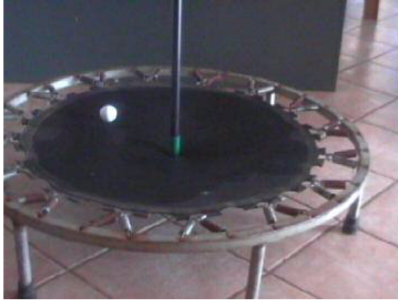
Figure 5: A mini-tramp is used as a gravitational potential well. A broom handle pushed down in the centre creates the necessary depression. A golf ball serves as the body in orbit.
